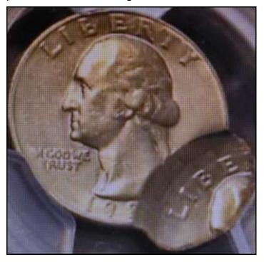
Today's high speed presses are capable of striking coins with four pairs of dies, with each pair striking around 700 coins per minute. If a struck coin is not properly pushed out of the chamber, another blank will be pushed in and you can have many, many possibilities. The struck coin can interfere with the striking of the new blank. The struck coin can act as a die and leave an incused impression on the new blank. At that point in time, you have a "mated pair".
