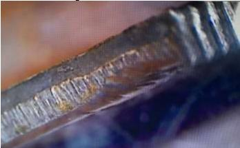
What makes this Kennedy half dollar neat is that the coin has a reeded edge, even inside the missing area. This totally bewilders me. It has always been my understanding that the reeding on a coin occured when the coin was struck and it expanded outward until it met the retaining collar, which pressed the reeding into the edge of the coin.
