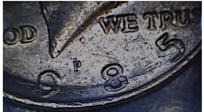
In conclusion, it is my belief that the obverse die had formed a die crack and under continued usage, the die broke. The retaining collar kept the two pieces together long enough for the press to continue striking cons, for a very short time. This is what guys that really know what's going on as a "terminal die state". The life of the usable die had ended.
